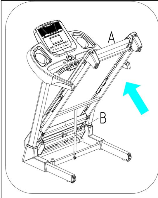
Place your hand at the end of the running deck (position A) and lift up the main frame (A02) until the air pressure cylinder (B03) locks (position B).
