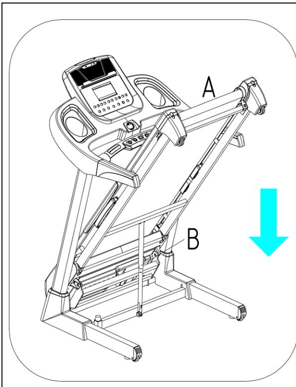
Grasp the main frame (A02) with one hand (position A) and use your foot to lightly kick the air pressure cylinder (B03) to unlock (position B). Give the main frame (A02) a downward push from position A and the running deck should automatically continue to steadily lower itself until the main frame (A02) reaches level ground.
